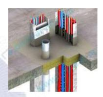
MEP Penetration: - Metal pipes, PVC pipes, Metal ducts, Insulated Metal Ducts (HVAC ducting, Grease duct).
